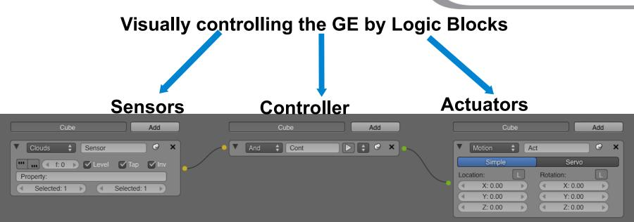
The GE system uses **Logic Blocks** as a visual way to set up **interactions** within the game. These logic blocks can be connected together visually to allow for complex game actions to take place.
