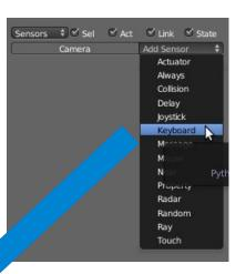
Add a **Keyboard** Sensor, an **And** Controller and a **Motion** Actuator
