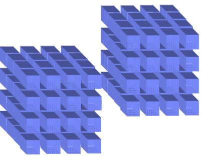
A midplane is 4x4x4x4x2 (512) nodes Sequoia full system is 16x16x16x12x2 nodes
