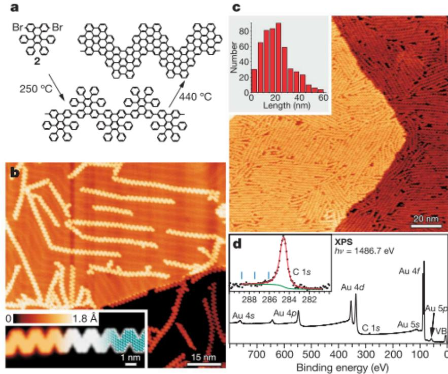
Figure 3 | Chevron-type GNRs from tetraphenyl-triphenylene monomers.
