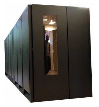
Computing nodes Processor: Xeon E5 2670 v2 (2.5 Ghz) Number of processors (cores): 1320 Number of nodes: 66 (20 cores per node) RAM: 128 GB/node
