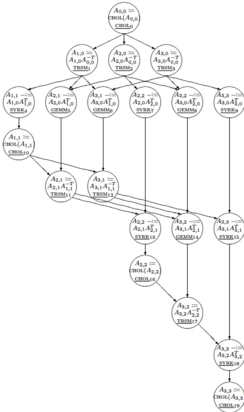
Figure 6.24: Graph of task dependencies in a 4 \times 4 Cholesky factorization
