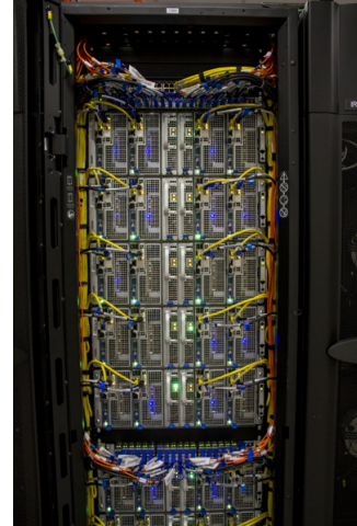
Figure 2.27: A fat tree with a three-level interconnect (left); the leaf switches in a cabinet of the Stampede cluster (right)
