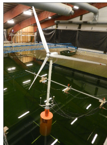
Laboratory tests on wind turbine with SPAR buoy and mooring system (EU-HYDRALAB-IV project, Tomasicchio et al.)
