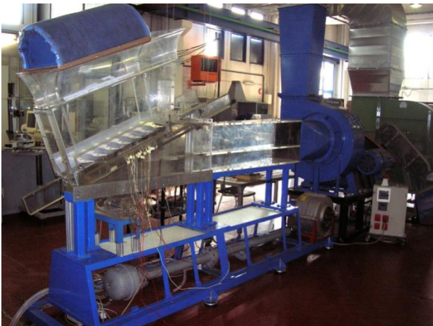
Suction-type, open circuit wind tunnel
