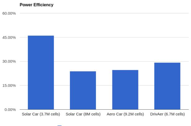
Power Efficiency GPU(S9150) vs CPU(12threads)
