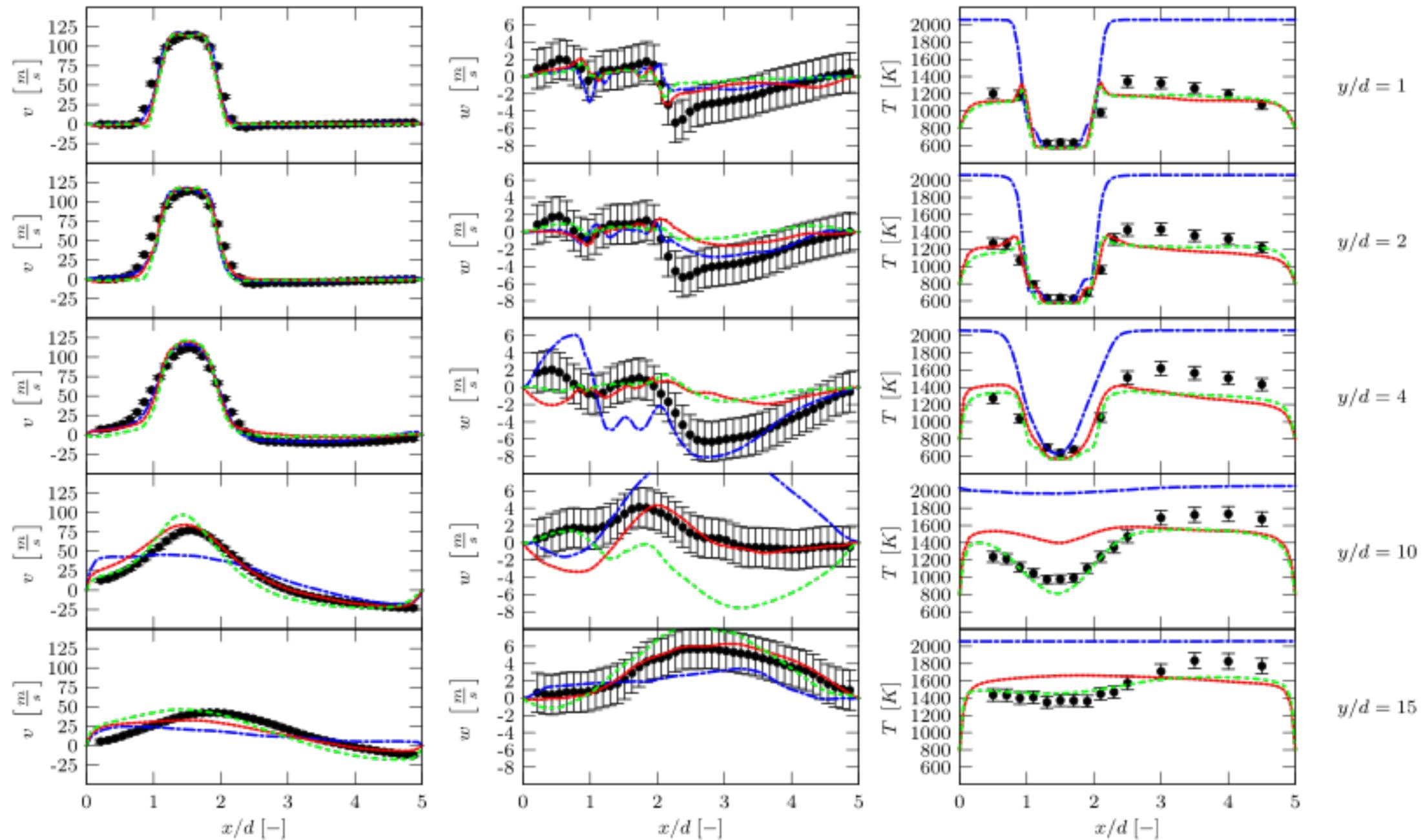
Profiles of time-averaged axial and transversal velocity and temperature for the LES simulations (dots: experiments, red: non-adiabatic, green: non-adiabatic with heat loss in chemistry).
