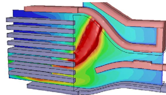
Circuit breaker (ANSYS Emag-ANSYS Fluent)
