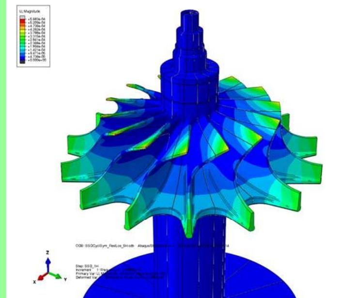
Blade vibrations due to pressure
