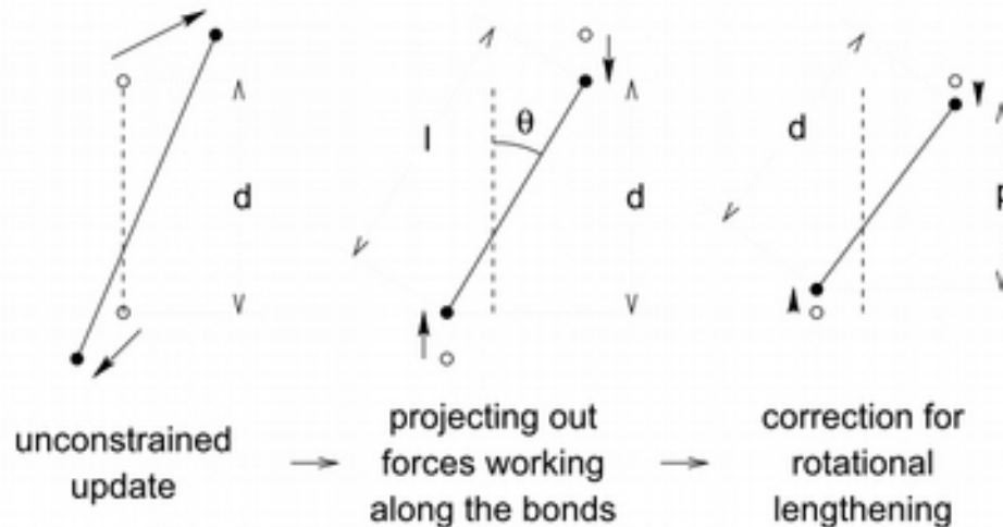
Figure 3.9: The three position updates needed for one time step. The dashed line is the old bond of length d , the solid lines are the new bonds. l = d \cos \theta and p = (2d^2 - l^2)^{\frac{1}{2}} .
