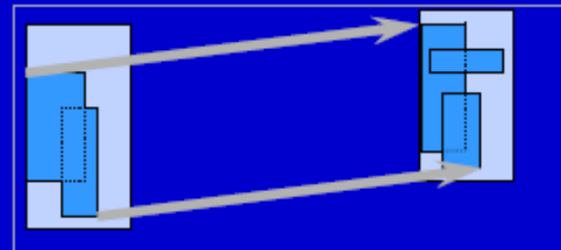
(d) Union of hyperslabs in file to union of hyperslabs in memory.
