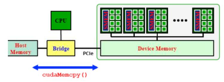
API blocking functions for data transfer between memories:
