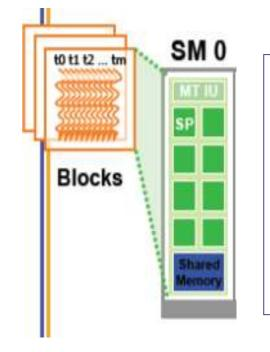
CUDA's hierarchy of threads/memories maps to the hierarchy of processors on the GPU:
